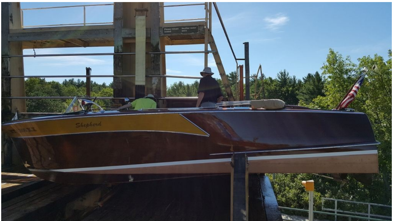
These two shots (above & below ) by Patti Bandi , show how inboard boats are loaded. Stem rests on deck, and a strap between two hydraulic posts supports bottom keeping strut and prop clear. Boat is positioned so strap lifts where coupler (transmission) and shaft meet.
